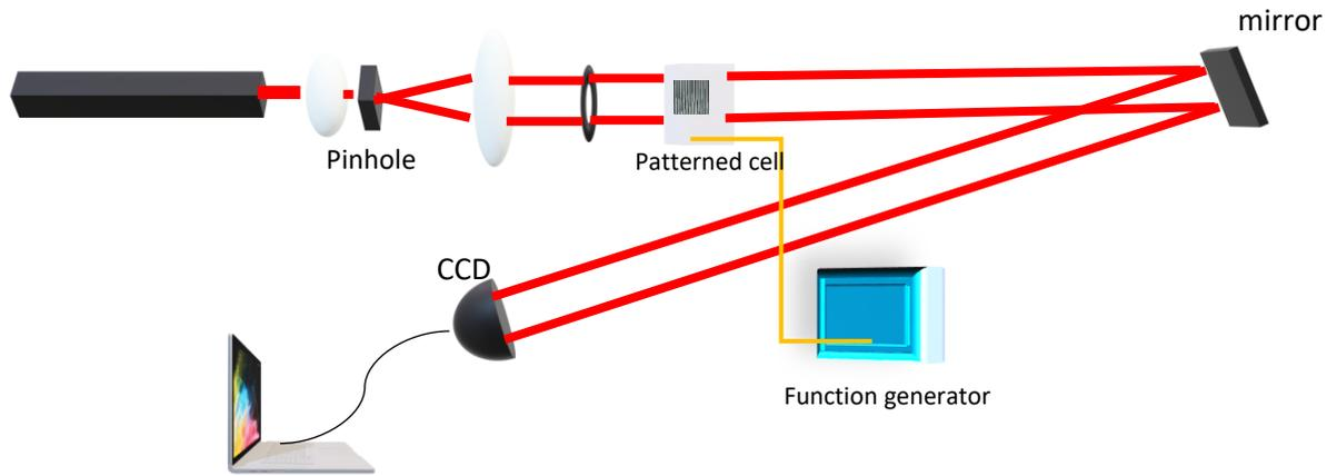
Figure 3: schematic diagram of generation vortex beam and controlling diffraction order
